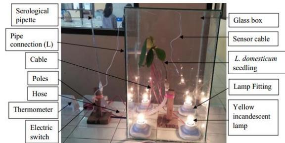
Fig. 1 Schematic of experimental tool
